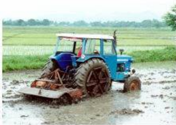
Creating a hard pan using a rotovator
