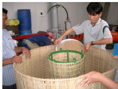
Figure 10: Construction of SRR-1 dryer with coal stove
