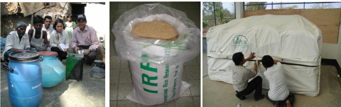
Figure 4: Hermetic storage systems made from locally available containers (left); the hermetic IRRI Super bag for 50kg (center); and a hermetic Cocoon™ with 5t capacity (right)
