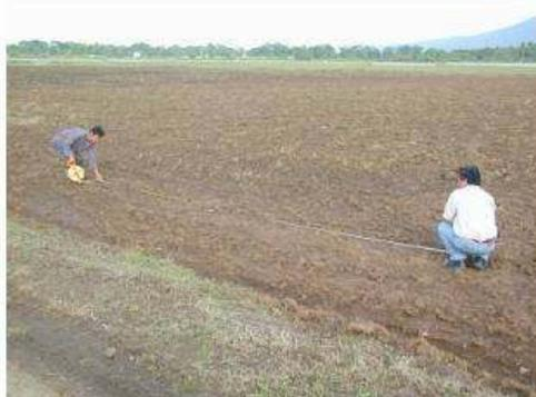
Steel tapes will be more accurate than other materials but can be less flexible and more prone to damage when being used.
