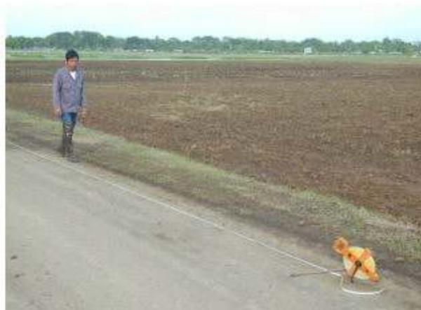
To calibrate a step, each individual must count the number of steps taken to walk a known distance in each environmental condition. This will vary according to the walking surface, the presence or otherwise of obstacles and the slope.
