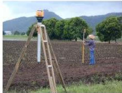
The laser transmitter transmits a laser beam, which is intercepted by the laser receiver mounted on the leveling bucket. The control panel mounted on the tractor interprets the signal from the receiver and opens or closes the hydraulic control valve, which will raise or lower the bucket.
