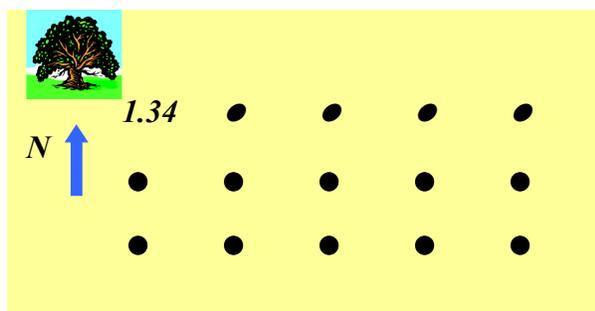
In the case of a land leveling exercise, where a cut/fill map is required, it is best to use the mean height of the field as a reference point. To determine the mean height of the field add together all of the measured points and divide by the number of measurements.
