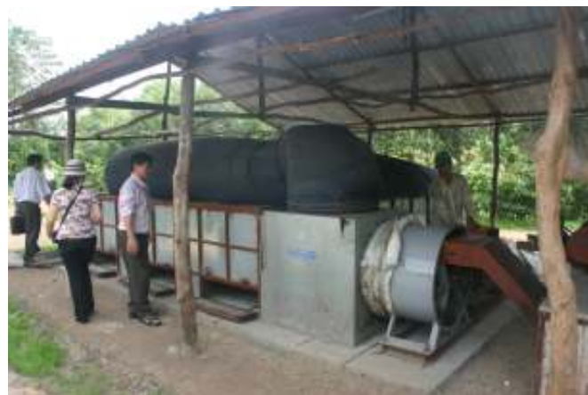
Figure 17: Principle (left) and example of a reversible-flow batch dryer in Vietnam using a canvas top and flaps in the plenum chamber to reverse the airflow (right)
