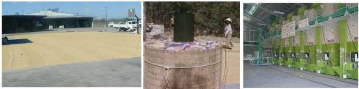
Figure 1: Sun drying pavement at a rice mill (left); farm level dryer in Vietnam (center); and re-circulating batch dryers at a rice mill
