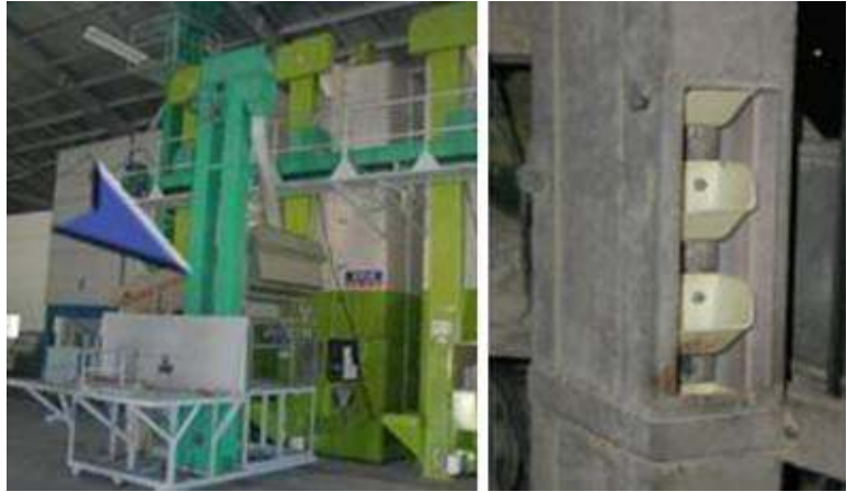
Figure 34: Bucket elevators on re-circulating batch dryers
