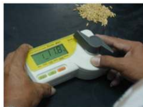
Figure 33: Commercial resistance type moisture meter
