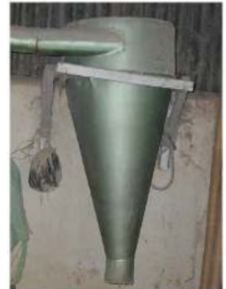
Figure 35: Simple cyclone for dust collection
